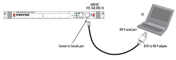
Figure 13. Connecting a serial terminal
